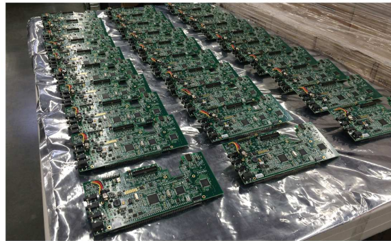
KX3 boards ready to move over to the burn-in rack for testing.
