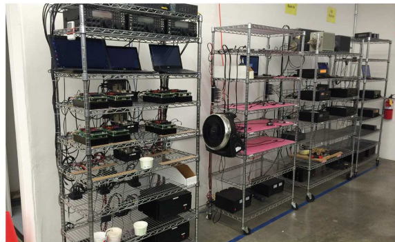
The burn-in area. Each Elecraft product is burned in and tested before it is shipped to make sure everything is operating up to spec.
